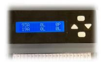
Prosense PEC Series Control Panel has three levels of alarm which are adjustable according to the measuring range and one fault alarm for the detection loop. Individual relays per function ensure remote controlled output. There are 5 relays on the panel. Three of them used as alarm relays and configured as ALARM-1, ALARM-2 and ALARM-3. There is one FAULT relay to monitor overall fault status. An additional relay programmed for optionally adjusted to alarm status.
