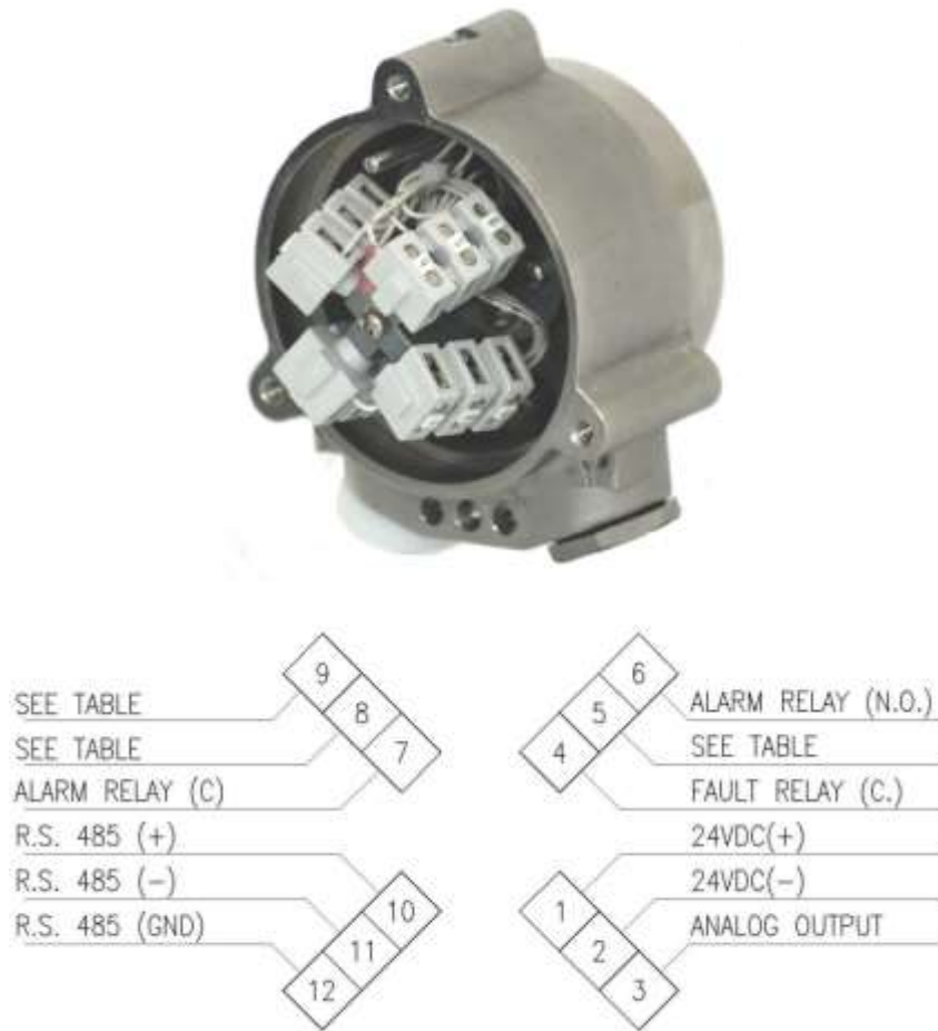
Figure 7: Wiring Terminals
