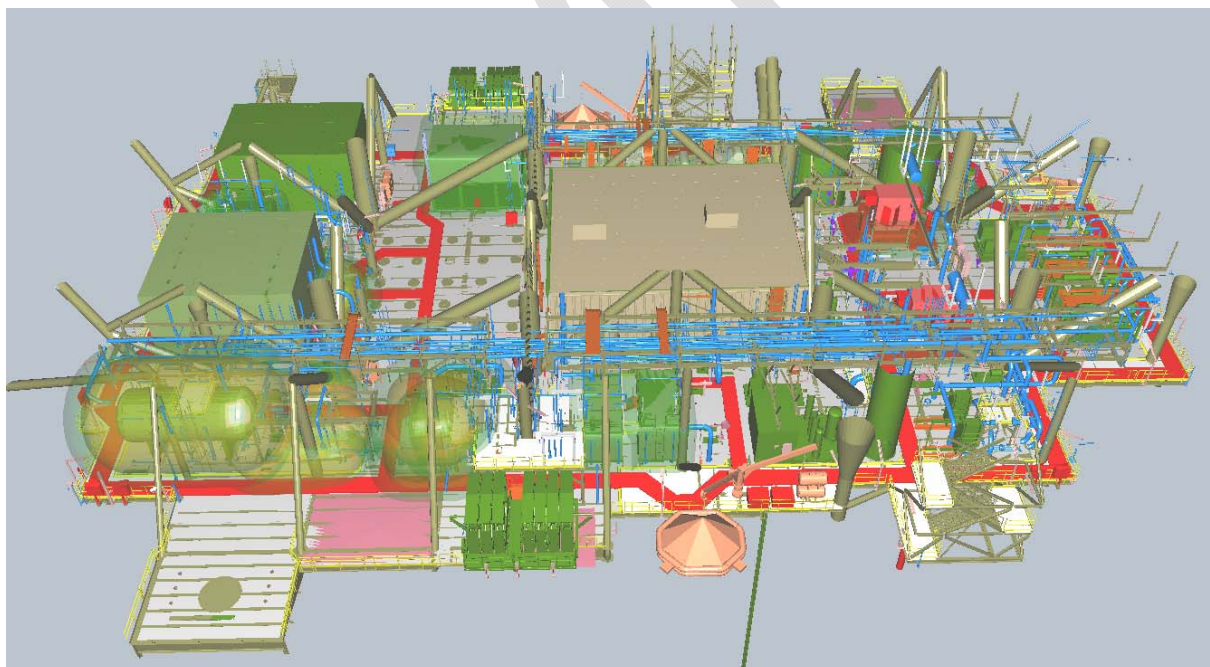
Figure 7.2.1.1: Screenshot showing the fire grademap throughout the Cellar deck within HazMap3D.
